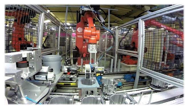
Robotic line for dispensing and dimensional control of the silicone curb with an accuracy of 0.2 mm
