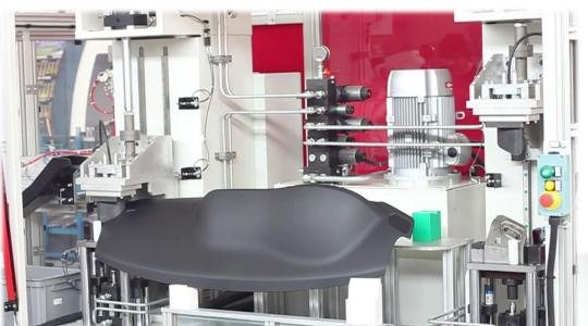
FCA trimming workcell on finished aesthetic piece. Accuracy of 0.05 mm.
