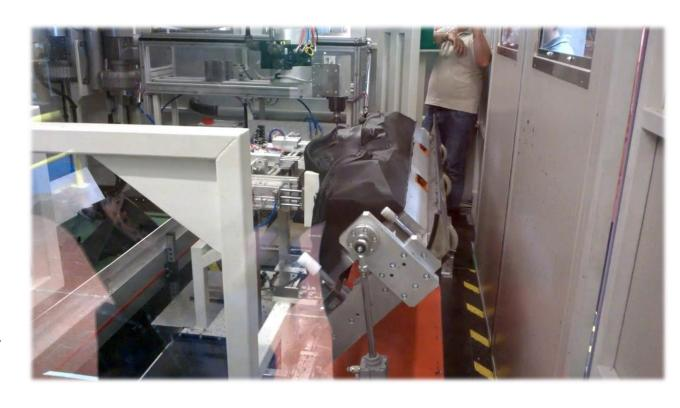
Robotized workcell for dashboard FCA milling with scrap removal and definition of the technician on the particular
