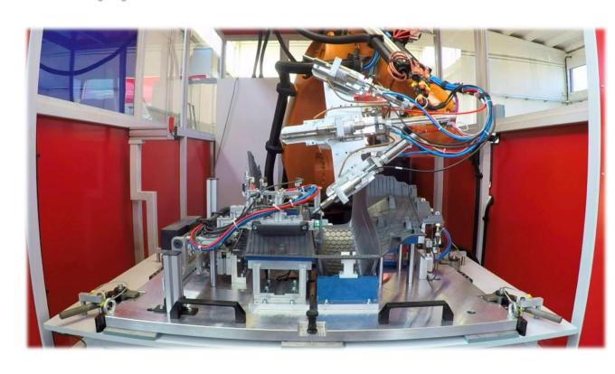
Robotized workcell for assembly of Caddy dashboard by ultrasonic welding, with interchangeable templates for more details.
